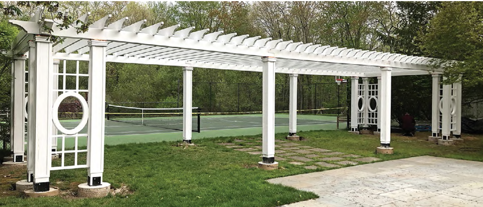
40' x 18' Custom Pergola with custom trellis panels between corner posts and custom copper caps on all posts.
