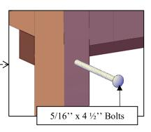
**Step 4:** Finally, use 5/16'' x  $3 \frac{1}{2}$ '' bolts (a) with washers and nuts to attach the diagonal supports (5) to the seat. After that, use 5/16'' x  $4 \frac{1}{2}$ '' bolts (b) with washers and nuts to attach to the legs. Each part has a series of numbers that indicate where to attach the part with the corresponding number.
