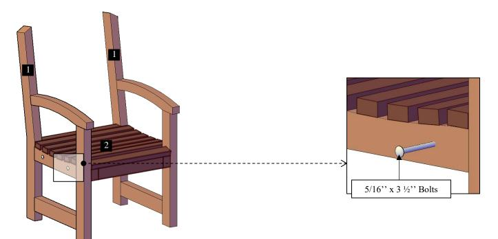
**Step 2:** Attach the backrest (3) to the legs with 5/16" x  $3\frac{1}{2}$ " bolts (a), washers and nuts. Each part has a series of numbers that indicate where to attach the part with the corresponding number.
