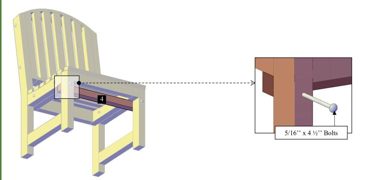
**Step 4:** Finally, use 5/16'' x  $3 \frac{1}{2}$ '' bolts (a) with washers and nuts to attach the diagonal supports (5) to the seat. After that, use 5/16'' x  $4 \frac{1}{2}$ '' bolts (b) with washers and nuts to attach to the legs. Each part has a series of numbers that indicate where to attach the part with the corresponding number.
