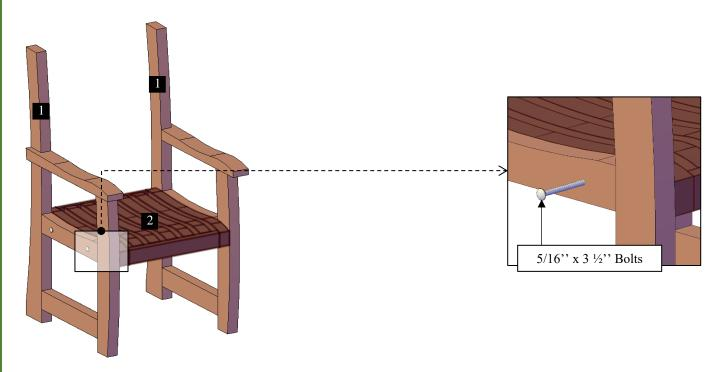
**Step 2:** Attach the backrest (3) to the legs with 5/16" x 3 ½" bolts (a), washers and nuts. Each part has a series of numbers that indicate where to attach the part with the corresponding number.
