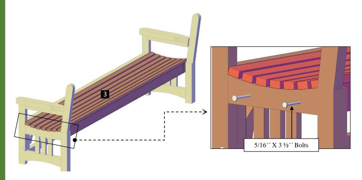
**Step 3:** Use  $5/16^{\prime\prime}$  x  $3\frac{1}{2}^{\prime\prime}$  bolts (**A**) to attach the seat (**3**) to the seat support. Each part has a series of numbers that indicate where to attach the part with the corresponding number.
