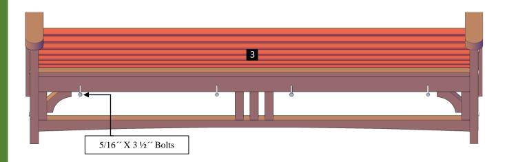
**Step 4:** Attach the backrest **(4)** to the legs with 5/16 x  $3\frac{1}{2}$  bolts **(A).** Each part has a series of numbers that indicate where to attach the part with the corresponding number.
