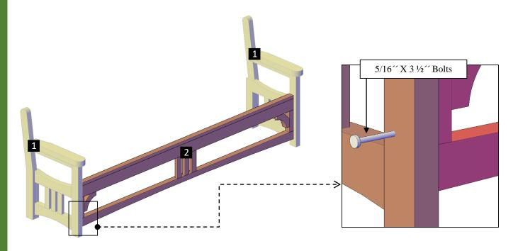
**Step 2:** Use 5/16" x  $3\frac{1}{2}$ " bolts (**A**) to attach the seat (**3**) to the legs. Each part has a series of numbers that indicate where to attach the part with the corresponding number.
