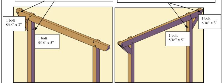
Repeat the same Steps, with the other posts, supports and roof timber. When you finish with these steps, you continue assembly the trellis walls.
