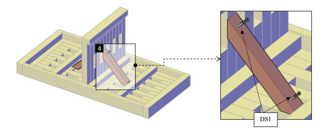
Step 3: Finally, use 5/16" x 3 ½" bolts (BL1) to attach the seat (1) to the Planter. Each part has a series of numbers that indicate where to attach the part with the corresponding number.
