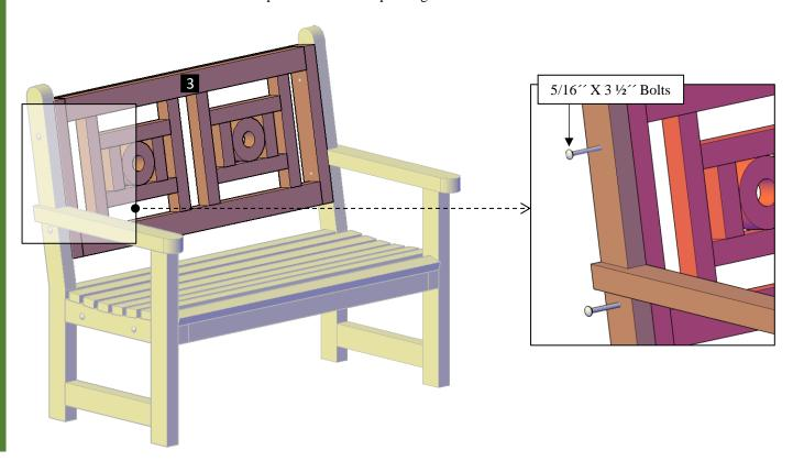
**Step 3:** Use 5/16 'x  $3\frac{1}{2}$ ' bolts (**A**) with washers (**C**) & nuts (**D**) to attach the diagonal supports (**4**) to the seat. After that, use 5/16 'x  $4\frac{1}{2}$ ' bolts (**B**) with washers (**C**) & nuts (**D**) to attach to the legs. Each part has a series of numbers that indicate where to attach the part with the corresponding number.
