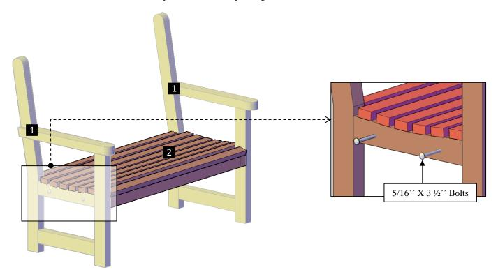
**Step 2:** Attach the backrest (3) to the legs, use 5/16" x 3 ½" bolts (A) with washers (C) & nuts (D). Each part has a series of numbers that indicate where to attach the part with the corresponding number.
