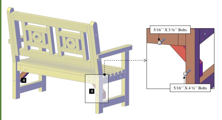
**Step 4:** Attach the support (5) to the legs, use  $5/16'' \times 4 \frac{1}{2}''$  bolts (B) with washers (C) & nuts (D). Each part has a series of numbers that indicate where to attach the part with the corresponding number.
