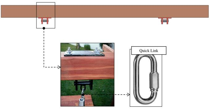
**Step 3:** Use 5/16" x  $3\frac{1}{2}$ " bolts (C) to attach support (3) to the posts. Each part has a series of numbers that indicate where to attach the part with the corresponding number.
