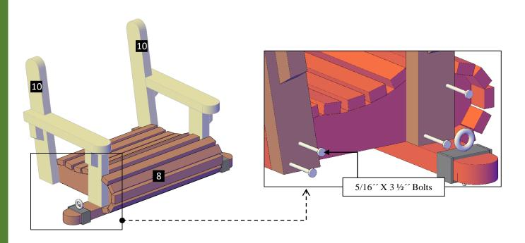
**Step 9:** Attach the backrest **(9)** to the armrest **(10)** with 5/16 "x 3 1/2" bolts **(C)** and 3/8" x 4" eyebolts **(I)**. Each part has a series of numbers that indicate where to attach the part with the corresponding number.
