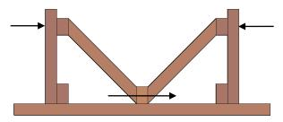
Small Benches – 1 bolt to attach each diagonal support to legs and 1 bolt to attach both diagonal supports to bench top
