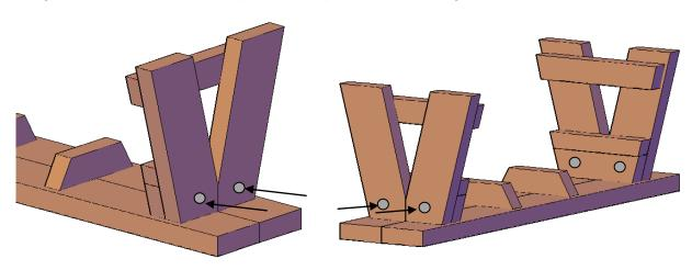
**Step 2:** Attach diagonal supports to legs and bench top. There are 3 cases to attach the diagonal supports and it will depend of your bench length. Match the numbers written next to the predrilled holes. If a hole is 5/16" then you must attach that part with a carriage bolt. For small benches you will notice that holes are tiny and you must attach the diagonal supports with deck screws provided for us.
