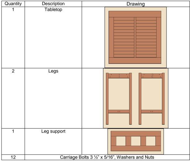
The parts that go together have the same numbers written next to the predrilled holes they attach to. Align the parts with the numbers as shown for ease of reference.
