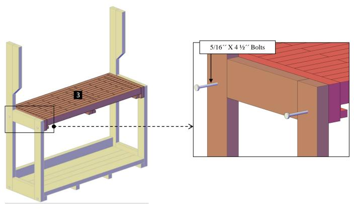
**Step 3:** Use 5/16" x 3 ½" bolts (**A**) to attach the top shelves (**4**) to the legs. Each part has a series of numbers that indicate where to attach the part with the corresponding number.
