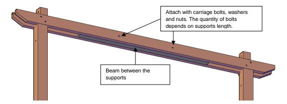
**Step 3.** Attach corner rafter to posts with one bolt per post (6 " x 3/8") washers & nuts. (Match numbers). Tap the bolt all the way into the wood to set it, then add a washer and nut and lightly tighten.
