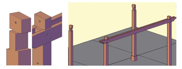
One the 2 supports have one large beam already attached or a few 18" pieces depending on size, this add support and strength to the structure. This beam must be in the interior of the support and bolted after you attach the supports to posts as shown below:
