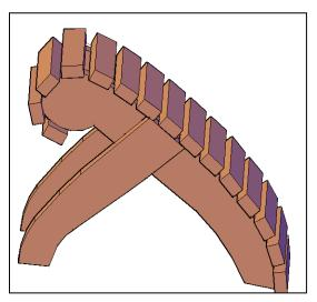
Make sure the bolts are tapped all the way into the wood, then add washers and nuts and tighten with a ½-inch ratchet. Do not over tighten or you'll crush the redwood and weaken the ottoman's structure.
