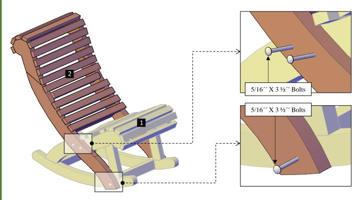
**Step 2:** Finally, attach the armrest (3) to the backrest with 5/16" x 3" bolts (**B**), washers (**C**) & nuts (**D**). After that, use 5/16" x 3 ½" bolts (**A**) with washers (**C**) & nuts (**D**) to attach the armrest to the seat. Each part has a series of numbers that indicate where to attach the part with the corresponding number.
