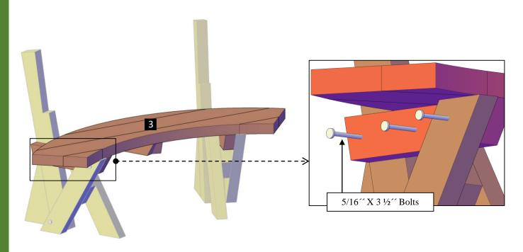
Step 3: Attach the diagonal supports (4) to the short legs and to the seat with 5/16" x 3 ½" bolts (B). Each part has a series of numbers that indicate where to attach the part with the corresponding number.
