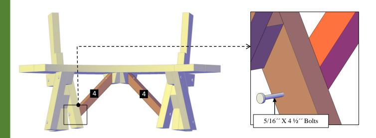
**Step 4:** Finally, use 5/16 ' x  $3\frac{1}{2}$  bolts (**B**) to attach the backrest (**5**) to the long legs. Each part has a series of numbers that indicate where to attach the part with the corresponding number.
