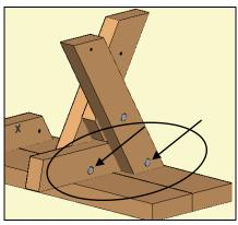
**Step 2:** Turn the bench over and attach back legs to seat with one bolt (3  $\frac{1}{2}$ " x 5/16"), washer & nut each one. Tap the bolt all the way into the wood to set it. Then add a washer and nut and lightly tighten.
