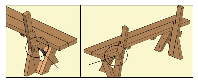
**Step 3:** Attach seat legs to back legs with one bolt (5  $\frac{1}{2}$ " x 5/16"), washer & nut each. Tap the bolt all the way into the wood to set it. Then add a washer and nut and lightly tighten
