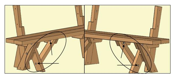
**Step 5:** Attach backrest to back legs, with two bolts (3½" x 5/16"), washers & nuts per side. Tap the bolt all the way into the wood to set it. Then add a washer and nut and lightly tighten.
