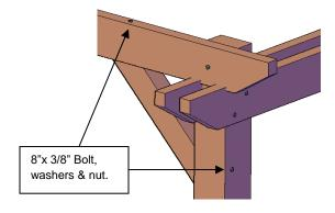
**Step 5.** Attach main knee brace to post & dual support beam with two bolts, washers & nuts. (Match numbers). Tap the bolt all the way into the wood to set it, then add a washer and nut and lightly tighten. Repeat this step with the other main knee braces.
