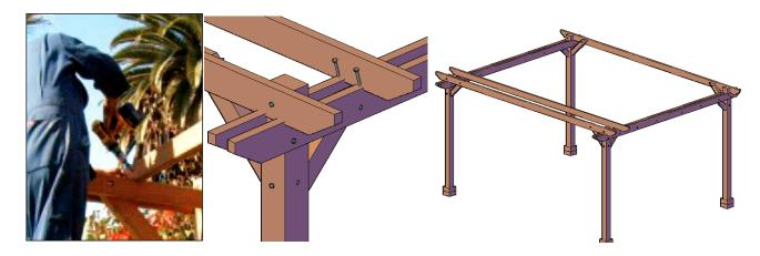
**Step 7.** Attach roof slats to rafters & with deck screws (3" x #8). The roof slats are all notched identically. The roof slats are notched to mesh with the rafters. The rafter tops are marked in ink every 18 inches with 2 lines. Place one roof slat into the lines on one end and begin to attach. *And repeat the process in all roof slats*.
