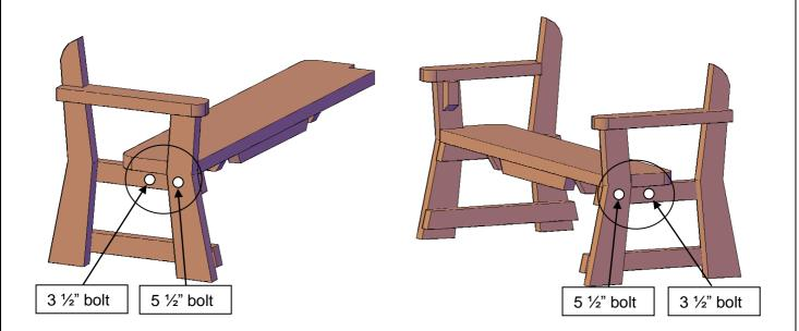
**Step 2:** Attach backrest to sides with 2 carriage bolts, washers and nuts per side. The backrest also has predrilled holes on each edge. Match the numbers to the predrilled holes on the side pieces. Tap in the  $3\frac{1}{2}$ " carriage bolts to attach the seat to the bench side. Tap the bolts in all the way, then insert the washer and nut and tighten with a  $\frac{1}{2}$ -inch ratchet. Do not over tighten or you'll crush the redwood and weaken the bench structure. Repeat for other side.
