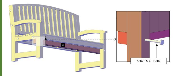
**Step 4:** Finally, use 5/16 'x  $3\frac{1}{2}$  'bolts (**A**) to attach the diagonal supports (**5**) to the seat. After that, use 5/16 'x 4 'bolts (**B**) to attach to the legs. Each part has a series of numbers that indicate where to attach the part with the corresponding number.
