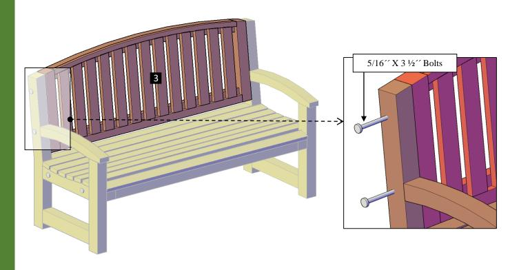
**Step 3:** Attach the frontal support (4) to the legs with  $5/16^{\prime\prime}$  x  $4^{\prime\prime\prime}$  bolts (B). Each part has a series of numbers that indicate where to attach the part with the corresponding number.
