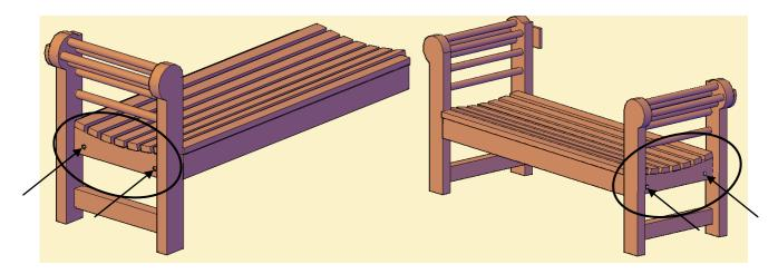
**Step 2:** Attach the backrest to side with two carriage bolts (5" x 5/16), washers and nuts. Match the numbers written next to the holes on both pieces. Tap the carriage bolt from the outside in. Tap the bolt in all the way, then add washers, nuts and tighten with  $\frac{1}{2}$ -inch ratchet. Do not over-tighten. Repeat this step to attach the backrest to the other side of the bench.
