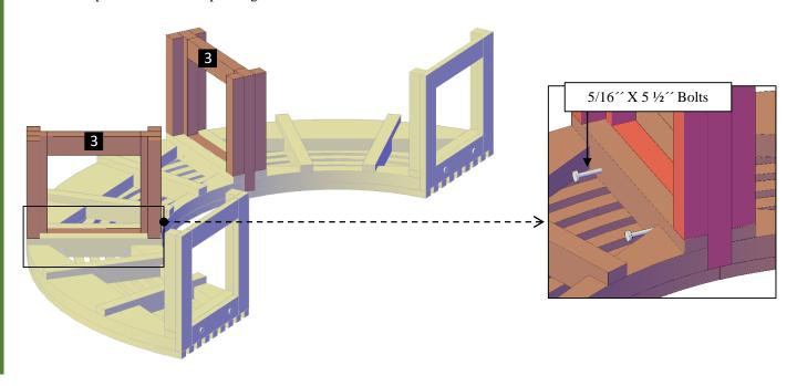
**Step 3:** Use 2 ½′′ deck screws **(C)** to attach the knee braces **(4)** to the seats and to legs. Each part has a series of numbers that indicate where to attach the part with the corresponding number.
