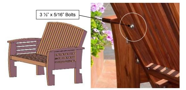
**Step 3**: Attach front support to sides with 2 bolts ( $4 \frac{1}{2}$ " x 5/16" Bolts) per side as shown below. Match the numbers next to the predrilled holes on the side's notch to the numbers on the back front support on each chair side. Tap the carriage bolts all the way into the wood, then attach the washers, nuts and tighten with  $\frac{1}{2}$ -inch ratchet. Do not over-tighten. Repeat this step to attach rear support.
