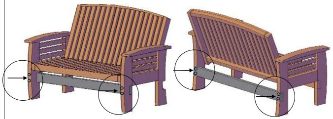
**Step 4**: Attach diagonal support to side and rear support with 2 bolts ( $3 \frac{1}{2}$ " x 5/16" Bolts), washers and nuts. Match the numbers next to the predrilled holes on the interior of the sides to the numbers on the rear support. Tap the carriage bolts all the way into the wood, then attach the washers, nuts and tighten with  $\frac{1}{2}$ -inch ratchet. Do not over-tighten. Repeat this step for the other diagonal support.
