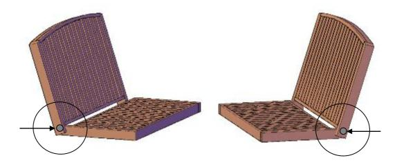
**Step 2**: Attach sides to backrest & seat. Each side has a groove on the inside of the frame for both the seat and the backrest to independently slide within.
