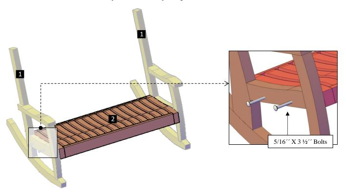
**Step 2:** Attach the backrest (3) to the legs with 5/16'' x  $3\frac{1}{2}''$  bolts (A), washers (C) & nuts (D). Each part has a series of numbers that indicate where to attach the part with the corresponding number.
