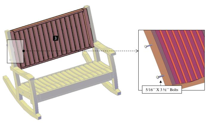
**Step 3:** Use 5/16 'x  $4\frac{1}{2}$ ' bolts **(B)** with washers **(C)** & nuts **(D)** to attach the support **(4)** to the legs. Each part has a series of numbers that indicate where to attach the part with the corresponding number.
