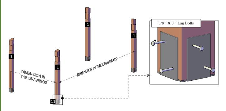
**Step 2:** First attach the single supports (2) to the posts (1) with 3/8 " X 11  $\frac{1}{2}$ " bolts (C). Each part has a series of numbers that indicate where to attach the part with the corresponding number.
