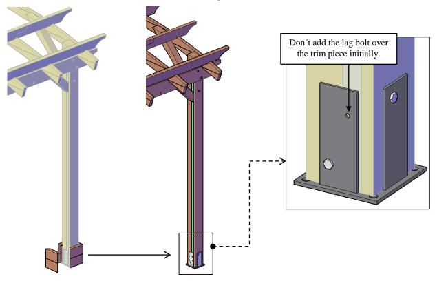
Step 2: Loosen the nut on the bolt support.
