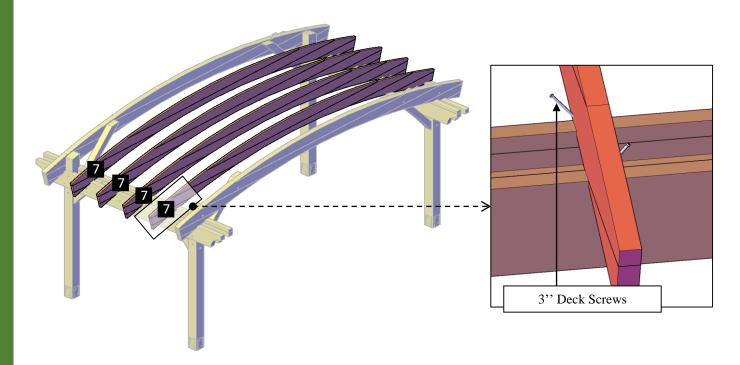
**Step 9:** Use 8" x 3" deck screws (**E**) to attach the Slats-A (**8**) and the Slats-B (**9**) to the arched rafters. Each part has a series of numbers that indicate where to attach the part with the corresponding number.
