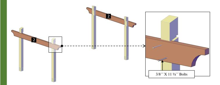
**Step 3:** Place the supports with in-between blocking (3), into the post notches as shown and attach to the posts with the single support bolts (C). Each part has a series of numbers that indicate where to attach the part with the corresponding number.
