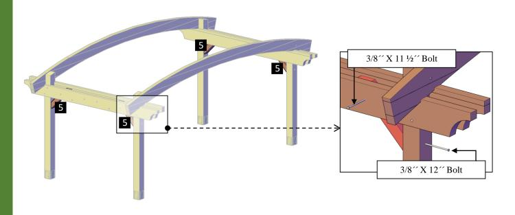
**Step 7:** Attach the secondary knee braces **(6)** to the posts with 3/8" x 12" bolts **(F)** and to the arched rafters with 5/16" x 8" bolts **(G)**. Each part has a series of numbers that indicate where to attach the part with the corresponding number.
