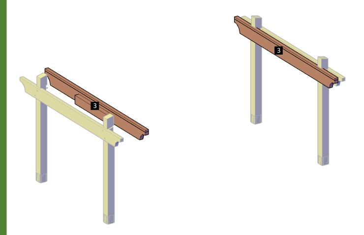
**Step 4:** Attach the single supports (2) to the supports with in-between blocking (3), use  $3/8^{\prime\prime}$  X 11  $\frac{1}{2}^{\prime\prime}$  bolts (C). The quantity of bolts depends on the length of the supports.
