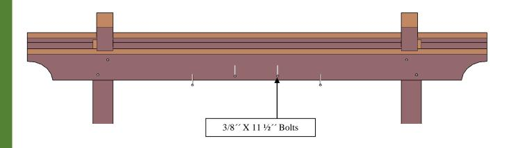
**Step 5:** Attach the perimeter arched rafters first (4) to the posts with 3/8" x 9  $\frac{1}{2}$ " bolts (**D**) and to the supports with 8" x 3" deck screws (**E**). Each part has a series of numbers that indicate where to attach the part with the corresponding number.
