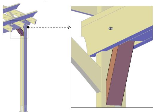
**Step 3:** The bolt of the post and the brace must be flush with the post.
