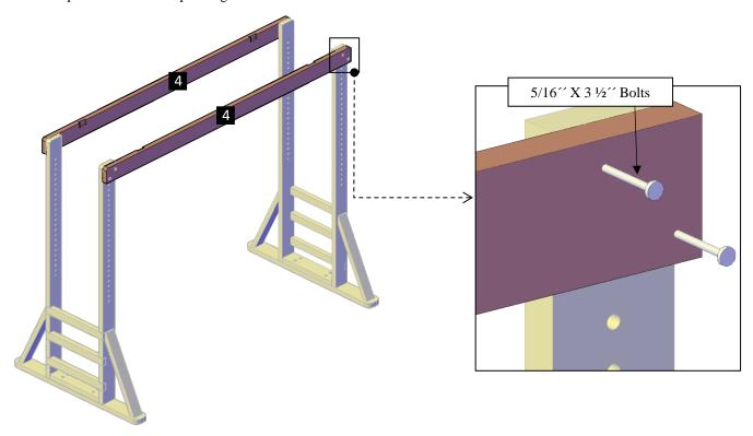
**Step 4:** Attach the knee Braces (5) to the legs and to the supports with  $5/16^{\prime\prime}$  x  $3\frac{1}{2}^{\prime\prime}$  bolts (A). Each part has a series of numbers that indicate where to attach the part with the corresponding number.
