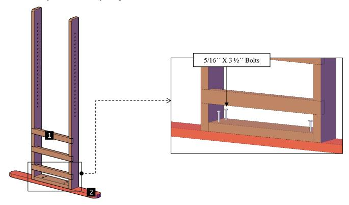
**Step 2:** Attach the diagonal supports (3) to the legs with 5/16" x 3" bolts (**B**) and to the leg bases with 5/16" x 3" bolts (**B**). Each part has a series of numbers that indicate where to attach the part with the corresponding number.
