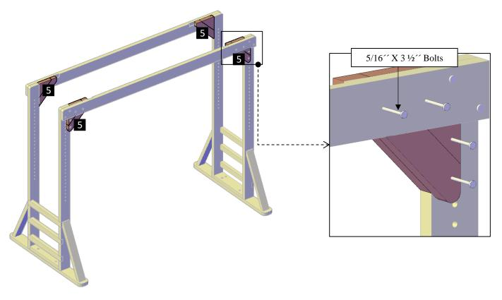
**Step 5:** Use 3"Deck Screws (**C**) to attach the top supports (**6**) to the supports. Each part has a series of numbers that indicate where to attach the part with the corresponding number.
