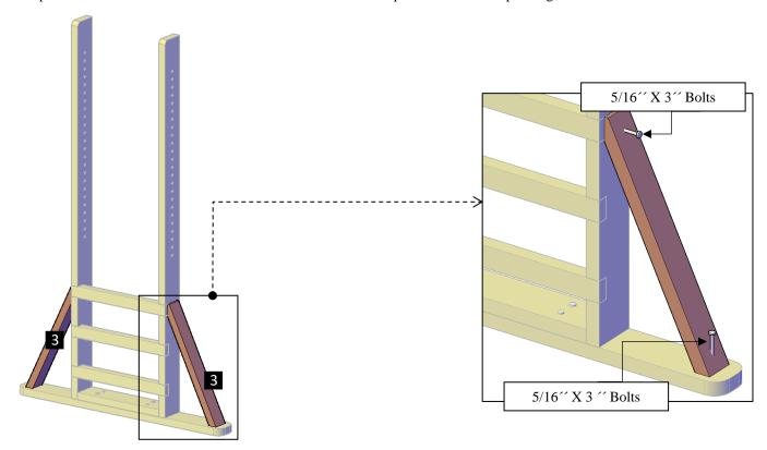
**Step 3:** Use  $5/16'' \times 3 \frac{1}{2}''$  bolts (A) to attach the supports (4) to the legs. Each part has a series of numbers that indicate where to attach the part with the corresponding number.
