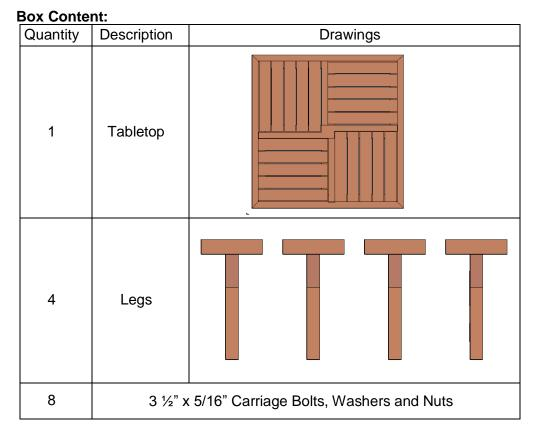
Your furniture was fully assembled in the shop prior to being dismantled for shipping. All the parts fit. The parts that go together have the same numbers written next to the predrilled holes they attach to. Please take the time to align the parts with the numbers. If you are forcing a bolt in, the part may be turned around or not aligned properly. Tap the bolt all the way into the wood to set it, then add a washer and lightly tighten. Don't over tighten or you will crush the redwood.
