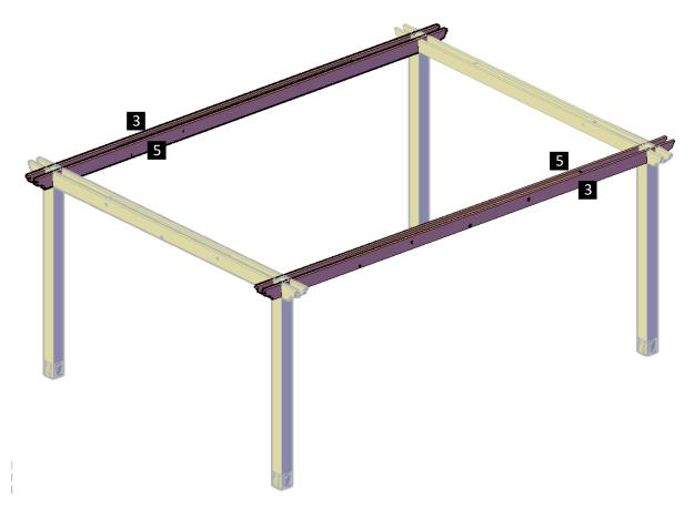
**Step 6:** Attach the secondary knee braces (9) and the main knee braces (8) to each posts with 3/8" x 12" bolts (**D**) with 3/8" washer (**G**) and 3/8 nut (**H**), and to the supports with 3/8" x 7 3/4" bolts (**C**) with 3/8" washer (**G**) and 3/8 nut (**H**). Each part has a series of numbers that indicate where to attach the part with the corresponding number.
