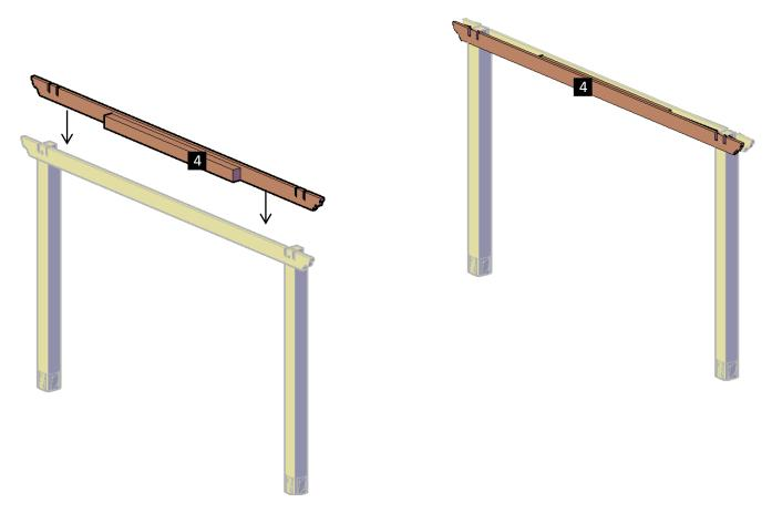
**Step 4:** Attach the short single supports (2) to the short supports with in-between blocking (4), use 3/8" X 7 3/4" bolts (C) with 3/8" washer (G) and 3/8 nut (H).
