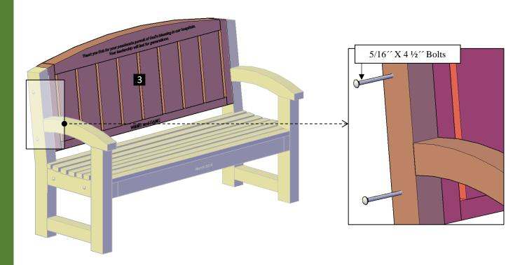
**Step 3:** Use 5/16" x  $5\frac{1}{2}$ " bolts (**B**) to attach the support (**4**) to the legs. Each part has a series of numbers that indicate where to attach the part with the corresponding number.
