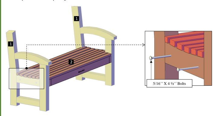
**Step 2:** Attach the backrest (3) to the legs with 5/16 x  $4\frac{1}{2}$  bolts (A). Each part has a series of numbers that indicate where to attach the part with the corresponding number.
