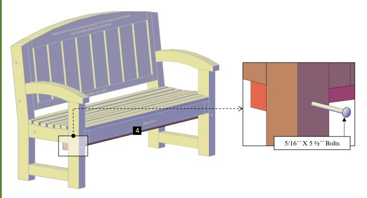
**Step 4:** Finally, attach the diagonal supports (5) to the seat with 5/16 x  $3 \frac{1}{2}$  bolts (C) and to the legs with 5/16 x  $5 \frac{1}{2}$  bolts (B). Each part has a series of numbers that indicate where to attach the part with the corresponding number.
