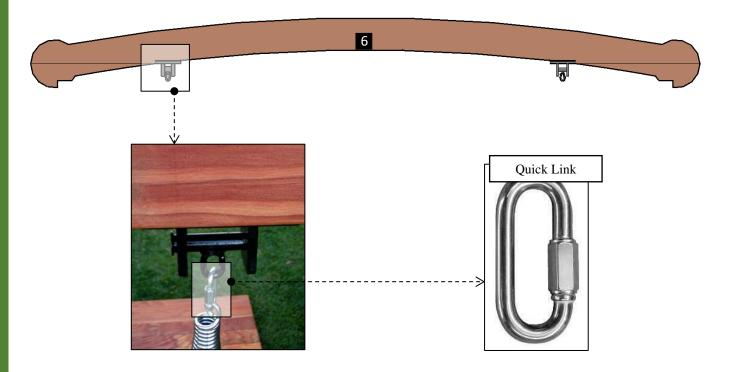
**Step 6:** Use 3/8 'x  $9\frac{1}{2}$ ' bolts (C) to attach the hanger support (6) to the legs-A. Each part has a series of numbers that indicate where to attach the part with the corresponding number.
