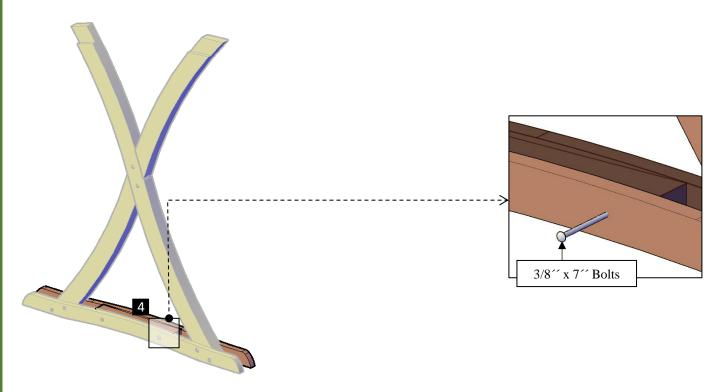
**Step 4:** Attach the top supports (5) to the legs with 3/8" x 7" bolts (B). Each part has a series of numbers that indicate where to attach the part with the corresponding number.
