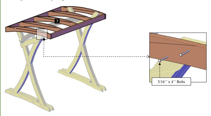
**Step 8:** Use 5/16 ' x  $4\frac{1}{2}$  ' bolts (**E**) to attach the diagonal supports (**8**) to the roof panel and 5/16 ' x 6 ' bolts (**F**) to attach to the legs. Each part has a series of numbers that indicate where to attach the part with the corresponding number.
