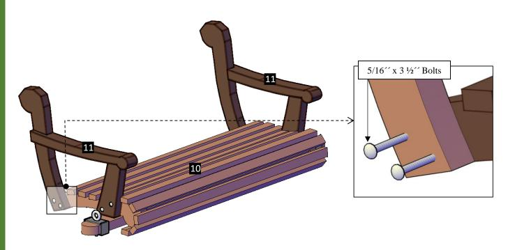
**Step 11:** Attach the backrest (12) to the armrests with 5/16" x 3 ½" bolts (A) and 3/8" x 3 ½" eyebolts (I). Each part has a series of numbers that indicate where to attach the part with the corresponding number.
