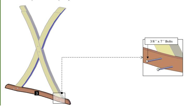
**Step 3:** Attach each bottom support with in-between blocking **(4)** to the legs with 3/8" x 7" bolts **(B)**. Each part has a series of numbers that indicate where to attach the part with the corresponding number.
