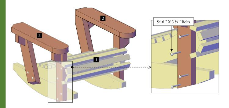
**Step 2:** Finally, attach the backrest (3) to the armrests, use 5/16 'x  $3\frac{1}{2}$  'bolts (A) with washers (B) & nuts (C). Each part has a series of numbers that indicate where to attach the part with the corresponding number.
