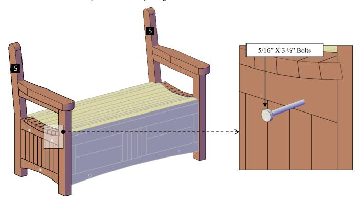
**Step 6:** Finally, use 5/16 'x  $3\frac{1}{2}$ ' bolts **(B)** to attach the backrest **(6)** to the legs. Each part has a series of numbers that indicate where to attach the part with the corresponding number.
