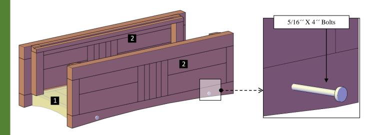
**Step 2:** Attach the short walls (3) to the long walls with  $5/16^{\prime\prime}$  x  $3\frac{1}{2}^{\prime\prime}$  bolts (B), as shown below. Each part has a series of numbers that indicate where to attach the part with the corresponding number.
