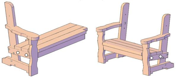
**Step 2:** Attach the backrest to sides with two carriage bolts (3 ½" x 5/16), washers and nuts per side. Match the numbers written next to the holes on each piece. Tap the carriage bolt from the outside in. Tap the bolt in all the way, then add washers, nuts and tighten with ½-inch ratchet. Do not over-tighten.
