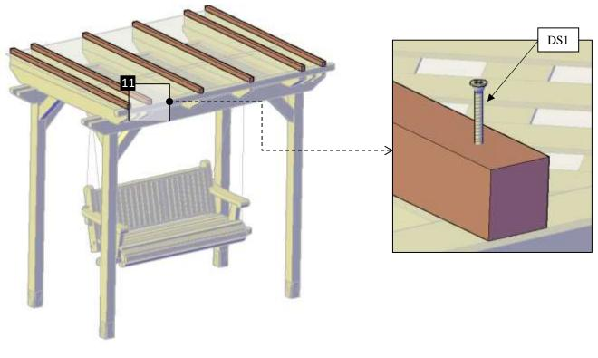
ANGEL'S TRELLIS SWING www.ForeverRedwood.com Step 17: Attach the slat (12) to the rafter top (11), use 3<sup>''</sup> deck screws (DS1). Check the marked numbers on each slat and place as drawings shown.
