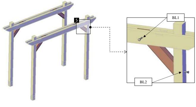
ANGEL'S TRELLIS SWING www.ForeverRedwood.com **Step 5:** Use 5/16" x  $5\frac{1}{2}$ " bolts (**BL3**) to attach the simple support-B (4) to the posts (1). Check the marked numbers on each simple support-B support and place as drawings shown.
