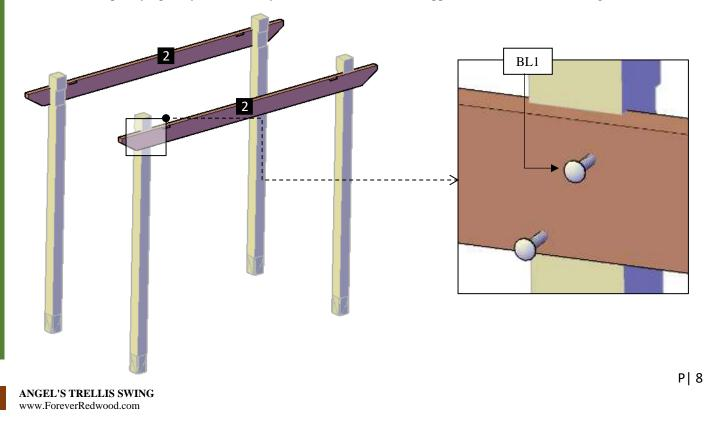
**Step 3:** Use 3/8" x 6 <sup>3</sup>/4" bolts (**BL1**) to attach the simple supports with in-between blocking-A (**3**) to the single support-A (**2**). Check the marked on each support with in-between blocking and place as drawings shown. *Note: return to the bolts described in the step 2 and tighten fully to attach in-between blocking to the post. Note: put silicone in the support with in-between blocking joins.*
