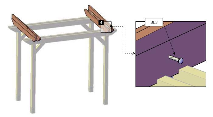
**Step 6:** Use 5/16" x  $5\frac{1}{2}$ " bolts (**BL3**) with washers & nuts to attach the secondary knee brace (6) to the secondary supports (4) and use 3/8" x 9" bolts (**BL2**) to the posts (1). Check the marked numbers on each secondary knee brace and place as drawings shown.
