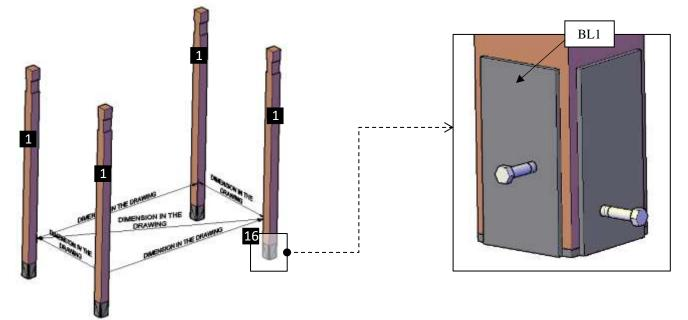
**Step 2:** Use 3/8" x  $6^{3}/4$ " bolts (**BL1**) to attach the simple support -A (2) to the posts (1). Check the marked numbers on each single support and place as drawings shown.
