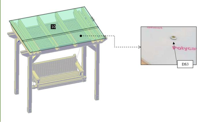
Step 15: Put exterior clear silicone on the polycarbonate joins.
