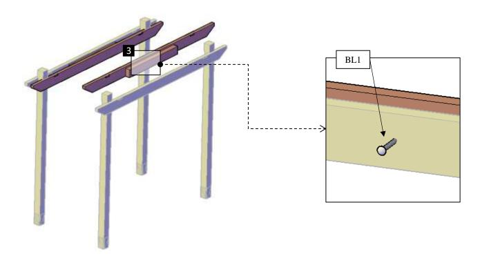
**Step 4:** Use 3/8" x 6 <sup>3</sup>/4" bolts (**BL1**) to attach the main knee brace (**5**) to the supports. After that use 3/8" x 9" bolts (**BL2**) to attach the main knee brace (**5**) to the posts (**1**). Check the marked numbers on each main knee brace and place as drawings shown.
