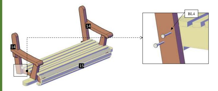
**Step 12:** Attach the backrest (13) to the arms with 5/16" x  $3\frac{1}{2}$ " bolts (**BL4**) with washer and nuts, and 3/8" x 4" eyebolts (**EB1**). Each part has a series of numbers that indicate where to attach the part with the corresponding number.
