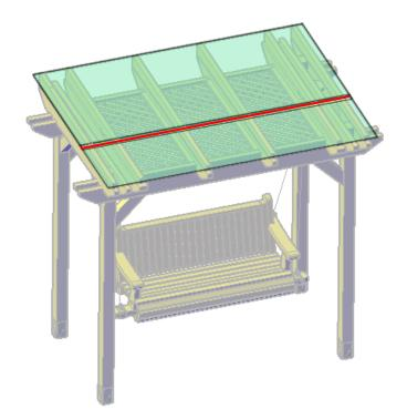
**Step 16:** Attach the rafter top (11) to the polycarbonate (10) & rafters (7), use 3<sup>---</sup> deck screws (DS1). Check the marked numbers on each rafter top and place as drawings shown.
