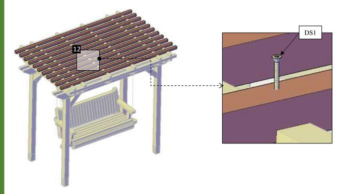
Step 18: Finally, use 3" deck screws (DS1) to attach the boot (17) to the posts (1).
