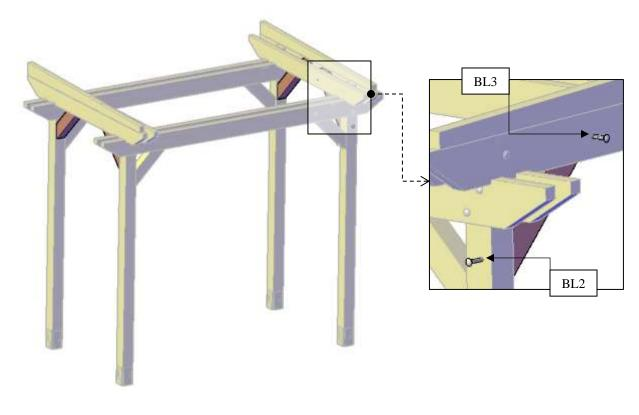
Step 7: Attach the rafter (7) to the supports with 3" deck screws (DS1). Check the marked numbers on each secondary knee brace and place as drawings shown.
