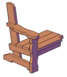
**Step 2:** Attach the Arm assembly left to the backrest, with two bolts ( $3 \frac{1}{2}$ " x 5/16"), washers & nuts. (Match up the numbers to attach the two parts together) Tap the bolt all the way into the wood to set it. Then add a washer and nut and lightly tighten. *Repeat this step with other side*.
