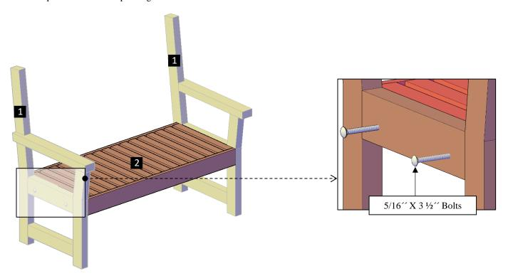
**Step 2:** Attach the backrest (3) to the legs with 5/16 ′′ x  $3\frac{1}{2}$  ′′ bolts (A). Each part has a series of numbers that indicate where to attach the part with the corresponding number.
