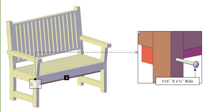
**Step 4:** Finally, attach the diagonal supports (5) to the seat with 5/16  $\times$  3  $\frac{1}{2}$  bolts (A) and to the legs with 5/16  $\times$  4  $\frac{1}{2}$  bolts (B). Each part has a series of numbers that indicate where to attach the part with the corresponding number.
