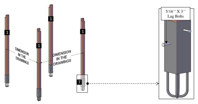
**Step 2:** Attach the supports (2) to the posts with 5/16" x 3  $\frac{1}{2}$ " bolts (C) washers & nuts. Tap the bolt all the way into the wood to set it. Then add a washer and nut and lightly tighten. Each part has a series of numbers that indicate where to attach the part with the corresponding number.
