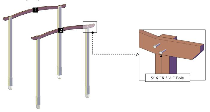
**Step 3:** Attach the knee braces (3) to the supports with 5/16" x  $3\frac{1}{2}$ " bolts (C) and to the posts with 5/16" x 5" bolts (D), washers & nuts. Each part has a series of numbers that indicate where to attach the part with the corresponding number.
