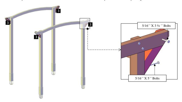
**Step 4:** Attach the trellis wall panels (4) to the posts with 5/16" x  $5\frac{1}{2}$ " bolts (**E**) washers & nuts. Each part has a series of numbers that indicate where to attach the part with the corresponding number.
