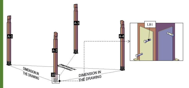
**Step 3:** Use 3/8" X  $6\frac{3}{4}$ " bolts (**BL1**) with washer and nuts to attach the single supports (2) to the posts. Check the marked on each support and place as drawings shown.
