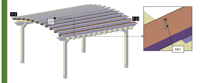
Step 12: Finally, attach the boots (9) to the posts with 3" deck screws (DS1).
