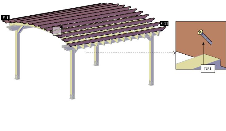
Step 10: Attach the arched reinforcement (8) to the arched rafters with 3<sup>''</sup> deck screws (DS1). Check the marked on each slat and place as drawings shown.
