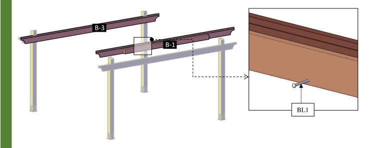
**Step 5:** Use 3/8" X 6" bolts (**BL2**) with washer and nuts to attach the perimeter arched rafter (**4**) to the posts and 3" deck screws (**D**) to attach to the supports. Check the marked on each perimeter arched rafter and place as drawings shown.
