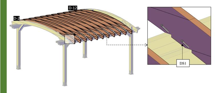
Step 10: Attach the slat (7) to the arched rafters with 3<sup>''</sup> deck screws (DS1). Check the marked on each slat and place as drawings shown.
