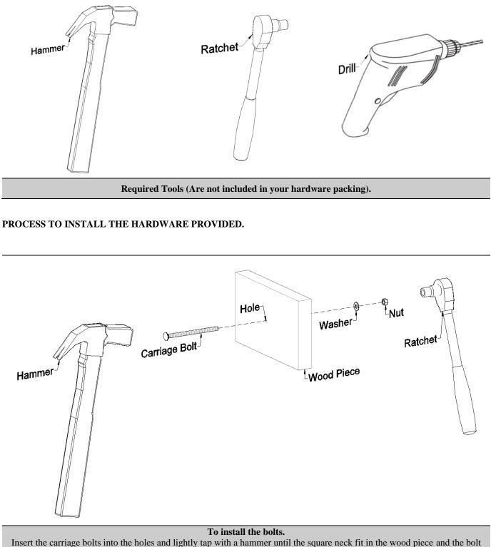
Insert the carriage bolts into the holes and lightly tap with a hammer until the square neck fit in the wood piece and the bolt head must flush with the wood piece. Finally, place the washer and the nut and carefully tighten it using a ratchet with the necessary socket or a wrench.
