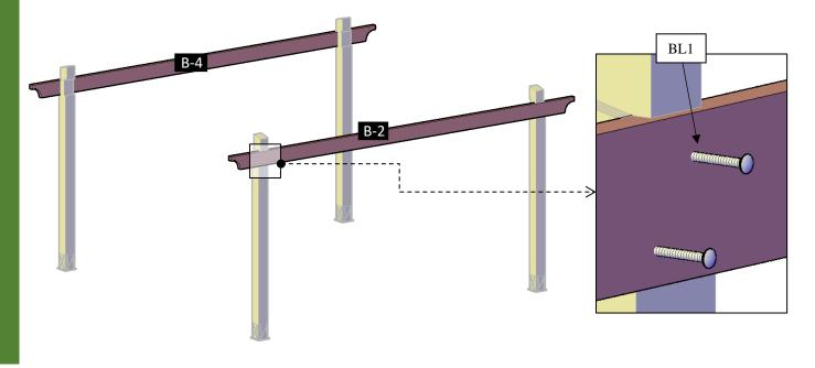
**Step 4:** Attach the single supports to the supports with in-between blocking (3), use 3/8" X 6 <sup>3</sup>/<sub>4</sub>" bolts (**BL1**) with washer and nuts. After that, return to the bolts described in the step 3 and tighten fully. Check the marked on each support with in-between blocking and place as drawings shown.
