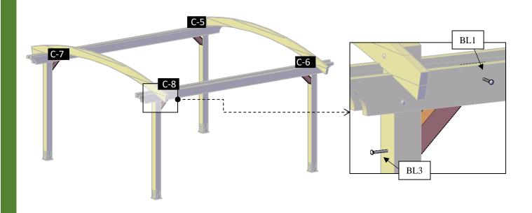
**Step 7:** Attach the Secondary knee braces (6) to the rafters with 3/8" X 5" bolts (**BL4**) with washer and nuts and to the posts with 3/8" x 9" bolts (**BL3**). Check the marked on each secondary knee brace and place as drawings shown.
