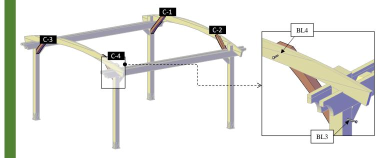
Step 8: Use 3<sup>''</sup> deck screws (DS1) to attach the arched rafters (4) to the supports. Check the marked on each arched rafter and place as drawings shown (D-2 at D-12).
