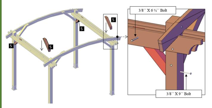
**Step 8:** Use 8" x 3" deck screws (**G**) to attach the other arched rafters (**4**) to the supports. Each part has a series of numbers that indicate where to attach the part with the corresponding number.
