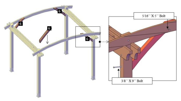
**Step 7:** Attach the main knee braces (5) to the posts with 3/8" x 9" bolts (**F**) and to the supports with 3/8" x 6 ½" bolts (**E**). Each part has a series of numbers that indicate where to attach the part with the corresponding number.
