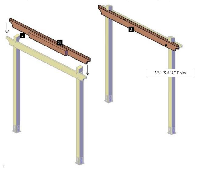
**Step 4:** Attach the single supports (2) to the supports with in-between blocking (3), use  $3/8^{\prime\prime}$  X  $6\frac{1}{2}^{\prime\prime}$  bolts (C). The quantity of bolts depends on the length of the supports.
