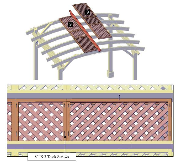
**Step 10.2:** Attach a slat (7,8) with 8" x 3" deck screw (G). Each part has a series of numbers that indicate where to attach the part with the corresponding number.
