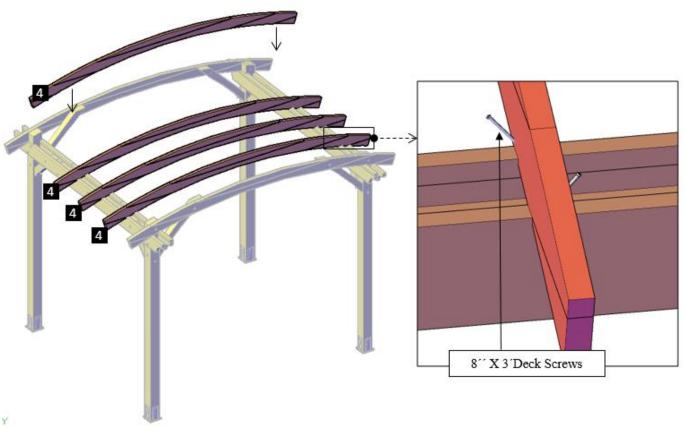
**Step 9:** Check you set of drawings and see if on the center top there is a roof lattice panel or a slat (7). You must attach this piece first with 8" X 3" deck screws (G). Each part has a series of numbers that indicate where to attach the part with the corresponding
