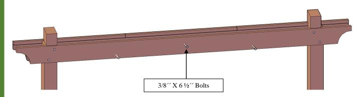
**Step 5:** Attach the perimeter arched rafters first (4) to the posts with 3/8" x 6" bolts (**D**) and to the supports with 8" x 3" deck screws (**G**). Each part has a series of numbers that indicate where to attach the part with the corresponding number.
