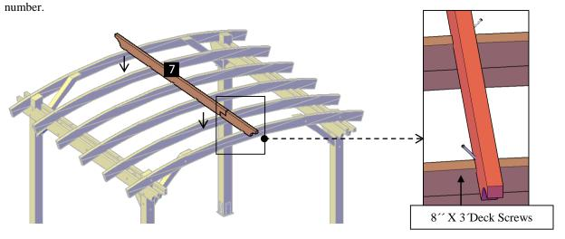
**Step 10:** Continue attaching the roof lattice panels (9) and the slats (7,8) to the arched rafters. Each part has a series of numbers that indicate where to attach the part with the corresponding number.
