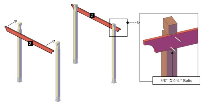
**Step 3:** Place the supports with in-between blocking (3), into the post notches as shown and attach to the post with the single support bolts. (C). Each part has a series of numbers that indicate where to attach the part with the corresponding number.
