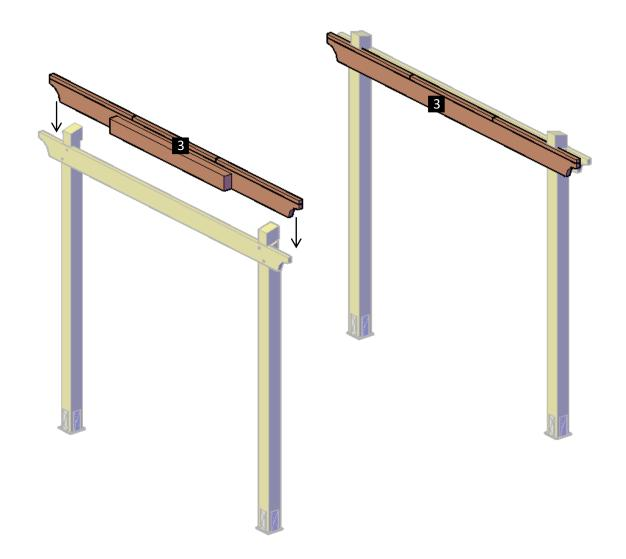
Step 4: Attach the single supports (2) to the supports with in-between blocking (3), use 3/8  $\times$  7  $\times$  bolts (C). The quantity of bolts depends on the length of the supports.
