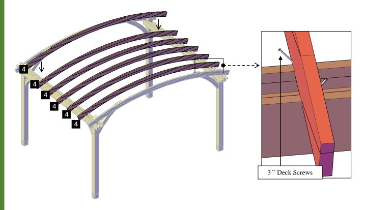
Step 9: Use  $15/8^{\prime\prime}$  deck screws (H) to attach the roof boards (7) to the arched rafters. Each part has a series of numbers that indicate where to attach the part with the corresponding number.
