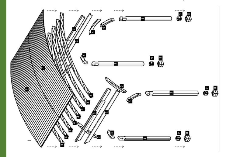
**NOTE:** In order to know where the post needs to be placed, check the numbers on them. If the post is not marked, then place the single Supports on the ground to locate the markings for each post position and clearly set your bearings. ("Don't attach yet, only place them on the ground to begin with").
