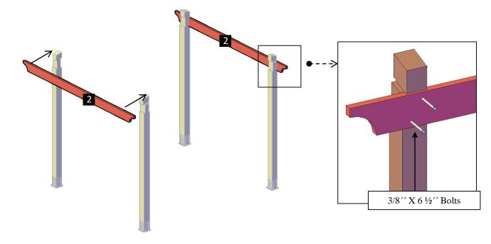
**Step 3:** Place the supports with in-between blocking (3), into the post notches as shown and attach to the posts with the single support bolts (C). Each part has a series of numbers that indicate where to attach the part with the corresponding number.
