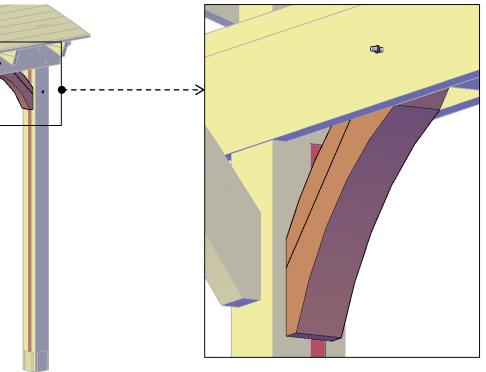
ARCHED THICK TIMBER PAVILION www.ForeverRedwood.com Step 3: The bolt of the post and the brace must be flush with the post.
