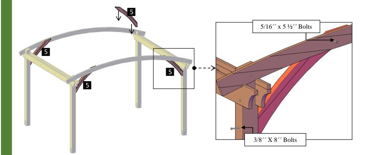
**Step 7:** Attach the main knee braces (6) to the posts with 3/8 x 8 bolts (E) and to the supports with 3/8 x 7 bolts (C). Each part has a series of numbers that indicate where to attach the part with the corresponding number.
