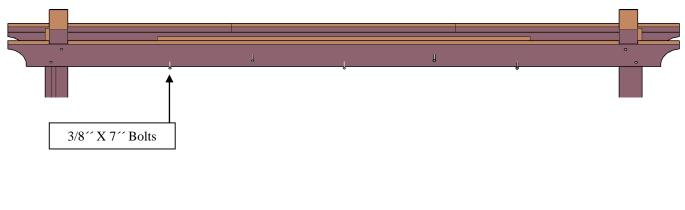
**Step 5:** Attach the perimeter arched rafters first (4) to the posts with 3/8 x 6 bolts (**D**) and to the supports with 8 x 3 deck screws (**G**Each part has a series of numbers that indicate where to attach the part with the corresponding number.
