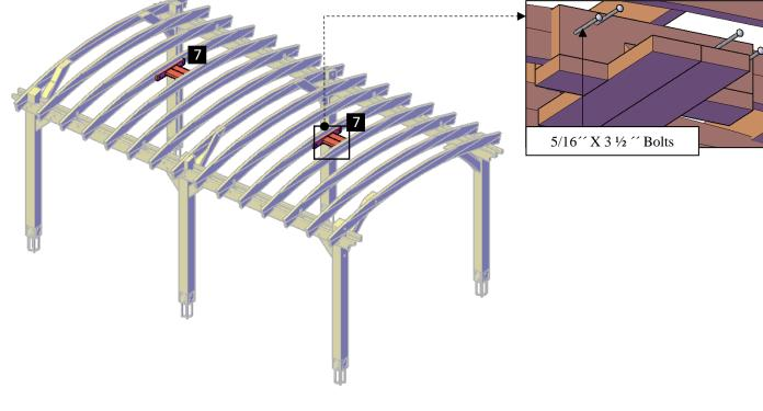
Step 10: Use  $1.5/8^{\prime\prime}$  deck screws (M) to attach the roof boards (8) to the arched rafters. Each part has a series of numbers that indicate where to attach the part with the corresponding number.
