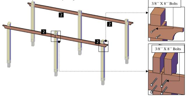
ARCHED THICK TIMBER PAVILION www.ForeverRedwood.com **Step 3:** Place the supports with in-between blocking (3), into the post notches as shown and attach to the posts with the single support bolts (C). Each part has a series of numbers that indicate where to attach the part with the corresponding number.
