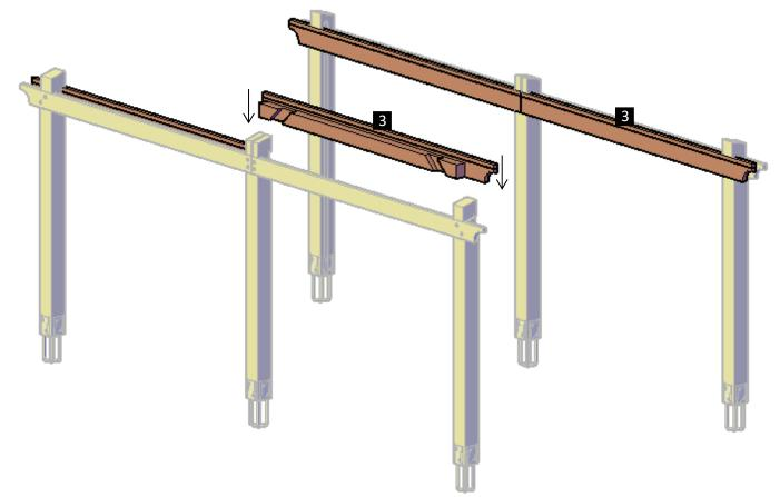
**Step 7:** First loosen the single support and place the main knee braces into the in-between blocking notches. Then, Attach the single main knee braces (4) to the posts with 3/8 ' x 12'' bolts (C) and the double main knee braces to the post with 3/8'' x 16'' bolts (D). Finally, use 3/8'' x 8'' bolts (B) to attach the main knee braces to the support.
