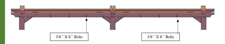
**Step 5:** Attach the perimeter arched rafters (5) to the posts with 3/8 x 7  $\frac{1}{2}$  bolts (E) and to the supports with 8 x 3 deck screws (G). After that, use 3/8 x 7 bolts (F) to attach the central arched rafter (5) to the post. Each part has a series of numbers that indicate where to attach the part with the corresponding number.
