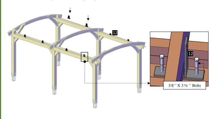
**Step 8:** Attach the rafters (5) to the hanger with 3/8 x  $1 \frac{1}{2}$  lag bolts (**I**) and to the supports with 3<sup> $\prime\prime$ </sup> deck screws (**G**). Each part has a series of numbers that indicate where to attach the part with the corresponding number.
