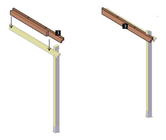
**Step 5:** Attach the single supports (2) to the supports with in-between supports (3), use 3/8 'X  $6 \frac{1}{2}$ ' bolts (C). The quantity of bolts depends on the length of the supports. Each part has a series of numbers that indicate where to attach the part with the corresponding number.
