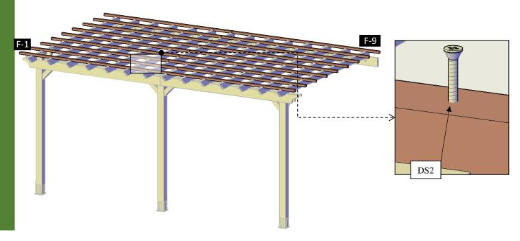
**Step 11:** Finally, attach the boots (10) to the posts with 3" deck screws (DS2).
