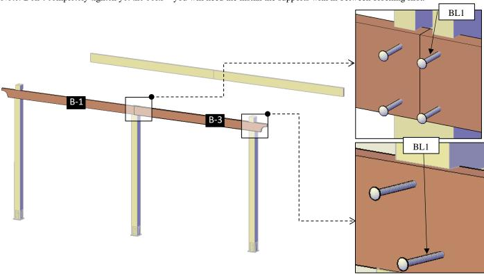
**Step 4:** Place the supports with in between blocking into the post notches. Return to the bolts described in the step 3 and tighten fully. After that use 3/8" x  $6\frac{1}{2}$ " bolts (**BL1**) to attach the supports together. Check the marked numbers on each support with inbetween blocking and place as drawings shown.
