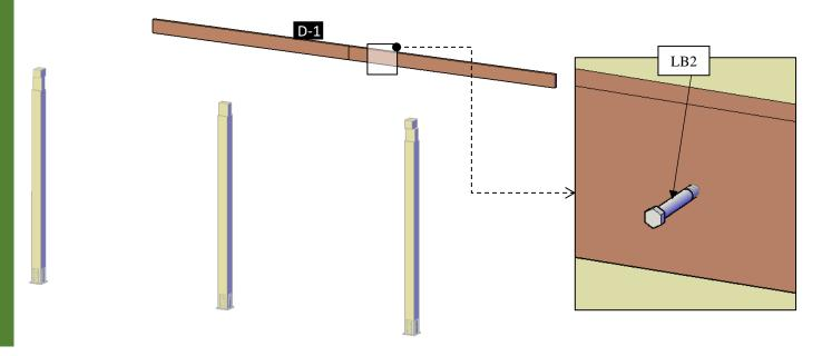
**Step 3:** Attach the single supports (3) to the posts with 3/8" x 6 ½" bolts (**BL1**) bolts with washers & nuts. Check the marked numbers on each support and place as drawings shown.
