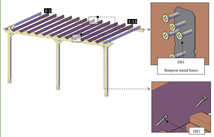
**Step 10:** Attach the slats **(8)** to the rafters with 3"deck screws **(DS2)**. Check the marked numbers on each slat and place as drawings shown (F-1 at F-9).
