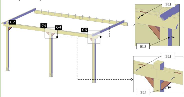
**Step 8:** Attach the secondary knee braces (7) to the Rafters with 5/16" x 5" bolts (**BL4**) and to the post with 3/8" x 9" Bolts (**BL3**) with washers & nuts. Check the marked numbers on each knee braces and place as drawings shown.
