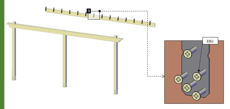
**Step 6:** Attach the Perimetral rafters (**5**) to the post with 3/8" x 6" bolts (**BL2**) with washers & nuts and use 3" deck screws (**DS2**) to attach to the supports and to the Simpson metal bases (**9**). Check the marked numbers on each rafter and place as drawings shown.
