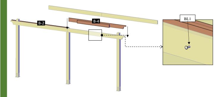
Step 5: Attach the Simpson metal bases (9) to the ledger board with 1 1/4" deck screws (DS1).
