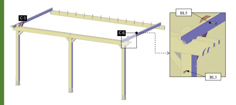
**Step 9:** Attach the rafters (5) to the supports with 3" deck screws (**DS2**) and to the Simpson metal bases (5) with 1 ¼" deck screws (**DS1**). Check the marked numbers on each rafter and place as drawings shown (E-2 at E-13).
