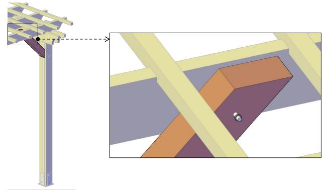
Step 3: The bolt of the post and the brace must be flush with the post.
