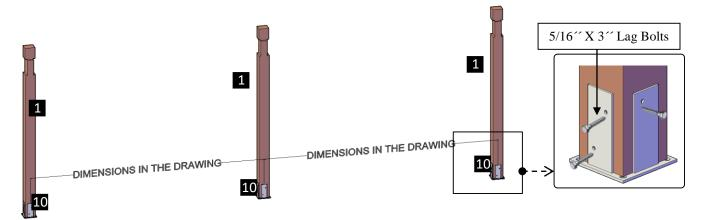
Step 2: Attach the wall mounted anchors (11) to the wall with  $\frac{1}{2}$  X 4<sup> $\prime\prime$ </sup> anchor bolts (G) (for concrete wall) or lag bolts (for wood wall).
