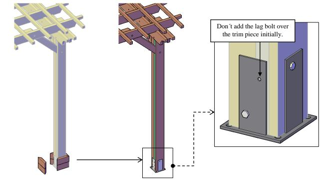
**Step 1:** First remove the deck screws to remove the boots of the post.
