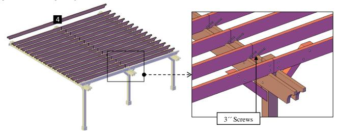
Step 9: Use  $3^{\prime\prime}$  screws (F) to attach the slats (7) to the rafters. Each part has a series of numbers that indicate where to attach the part with the corresponding number.
