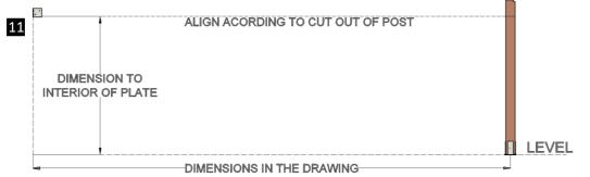
**Step 3:** First attach the single supports (2) to the posts with 3/8  $\times$  7  $\times$  bolts (A). After that, place the supports with in-between blocking (3), into the post notches as shown and attach to the posts with the single support bolts. Each part has a series of numbers that indicate where to attach the part with the corresponding number.
