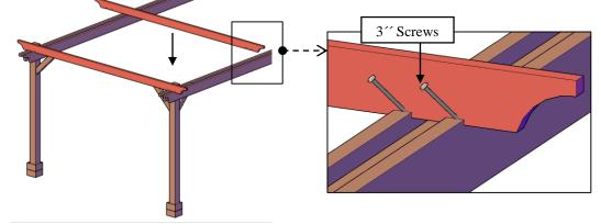
**Step 12:** Continue attaching the side panels and the rafters. Use the deck screws supplied. Attach the roof lattice panels (8) to the support and to the sides of the rafters. A screw every 2 or 3 feet is enough. Each part has a series of numbers that indicate where to attach the part with the corresponding number.
