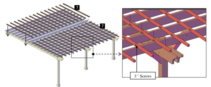
Step 10: Use 3" screws (F) to attach the boots (9) to the posts.
