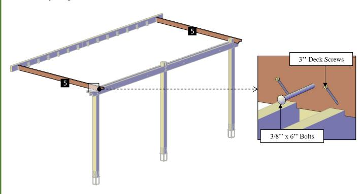
**Step 7:** Use 3/8" x 5 ½" bolt (**G**) to attach the central rafter (**5**) to the central post and 2" deck screws to attach to the joist hanger. Each part has a series of numbers that indicate where to attach the part with the corresponding number.
