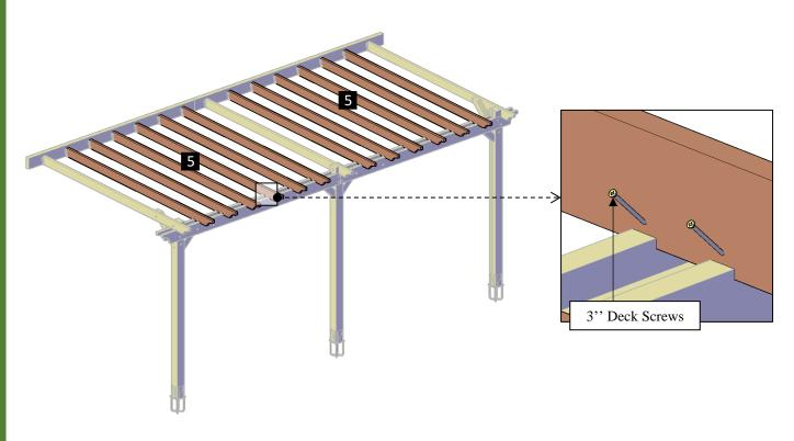
**Step 11:** Attach the slats **(8)** to the rafters with 3" deck screws **(F)**. Each part has a series of numbers that indicate where to attach the part with the corresponding number.
