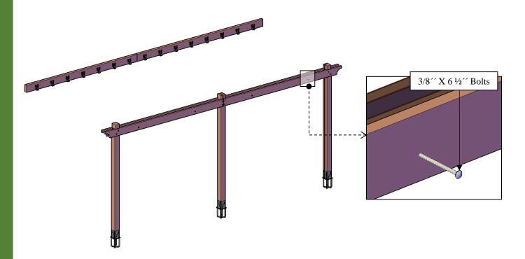
**Step 6:** Use 3/8" x 6" bolts (**E**) to attach the perimeter rafters (**5**) to the posts and 2" deck screws to attach to the joist hangers. After that, attach to the supports with 3" deck screws (**F**). Each part has a series of numbers that indicate where to attach the part with the corresponding number.
