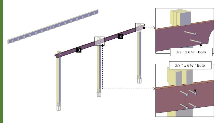
**Step 4:** Put up the supports with in-between blocking (4), into the post notches as shown and attach to the posts with the single support bolts. Each part has a series of numbers that indicate where to attach the part with the corresponding number.
