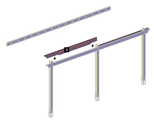
Step 5: Attach the single supports to the supports with in-between blocking, use 3/8" X 6 ½" bolts (**D**).
