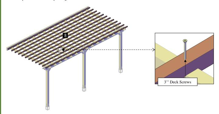
**Step 12:** Finally, use 3" Deck Screws (**F**) to attach the boots (**9**) to the posts. Each part has a series of numbers that indicate where to attach the part with the corresponding number.
