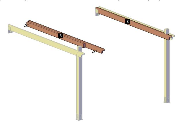
**Step 5:** Attach the single supports to the supports with in-between blocking, use 3/8  $^{\prime\prime}$  X  $6\frac{1}{2}$  bolts (**D**). The quantity of bolts depends on the length of the supports.
