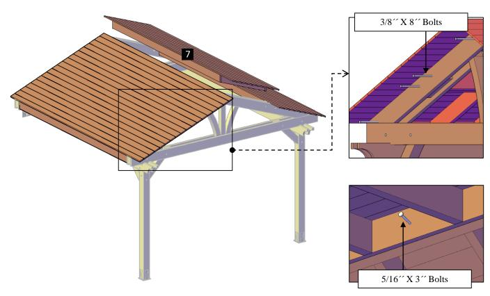
Step 12: Attach the roof panels (7) to the triangles with 2 1/4" deck screws (F).
