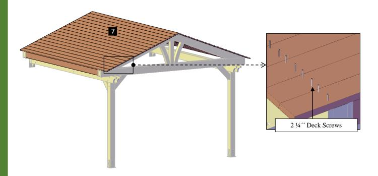
**Step 13:** Attach the roof fascia's **(8)** to the roof panels with 2 1/4" deck screws **(F)**. Each part has a series of numbers that indicate where to attach the part with the corresponding number.
