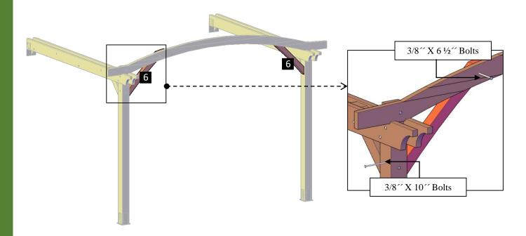
**Step 10:** Use 3" deck screws () to attach the rest of triangles (4) or arched rafters (4) to the supports. Each part has a series of numbers that indicate where to attach the part with the corresponding number.
