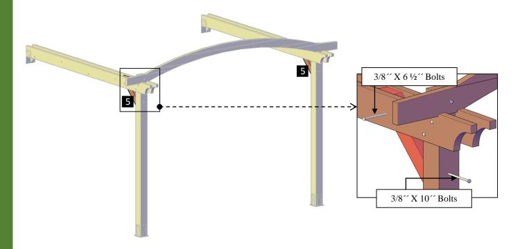
**Step 9:** Attach the secondary knee braces **(6)** to the posts with 3/8" x 10" bolts **(G)** and to the triangle or the arched rafter with 3/8" x  $6\frac{1}{2}$ " Bolts **(D)**. Each part has a series of numbers that indicate where to attach the part with the corresponding number.
