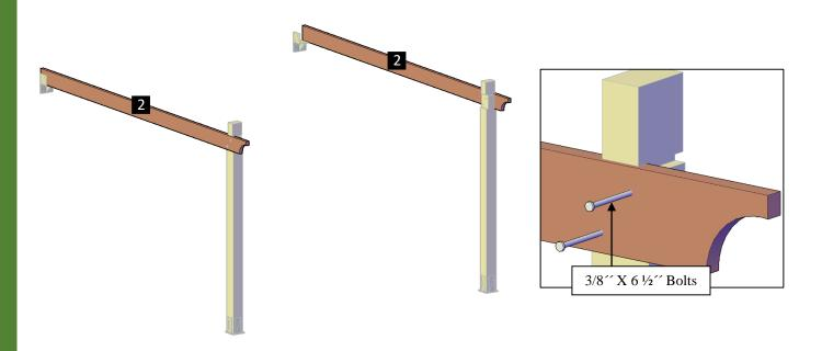
**Step 4:** Put up the supports with in-between blocking (3), into the post notches as shown and attach to the posts with the single support bolts. Each part has a series of numbers that indicate where to attach the part with the corresponding number.
