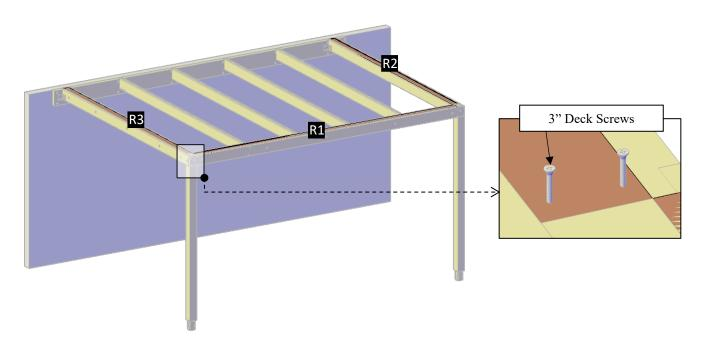
**Step 9:** Use 5/16" x 2 ½" lag bolts (**E**) to attach the L-Plaques (**13**) to the posts and to the Support and 3" Deck Screws (**I**) to attach to the Supports. Match the number in the angles with the number in the posts.
