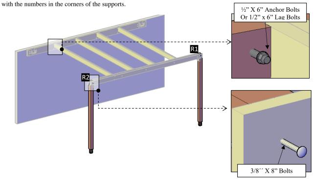
**Step 6:** Use 3/8" X 8" Bolts (**H**) to attach the Single Supports-B (**5**) to the posts. Match the number in the corners of the Supports with the numbers in the notches of the posts and the ledger boards.
