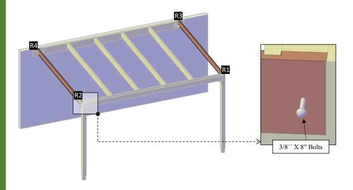
**Step 7:** Use 5/16" X 3" Lag Bolts (**B**) to attach the Supports Metal Plaques (**14**) to the Supports-B (**5**). After that, use 3/8" X 7" Bolts (**C**) to attach the Single Supports-B together. Match the number in the center of the supports.
