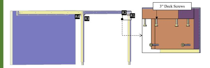
**Step 11:** Use 2" Deck Screws(**J**) or 2 ½" Deck Screws to attach the Bamboo Slats (**10**) to the Panel (**9**). \**Note: extra pieces (in case if necessary).*
