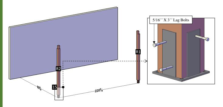
**Step 2:** Use 3/8'' X 7" bolts (**C**) to attach the Supports-A with in-between (**4**) to the supports. Match the number in the center of the supports.
