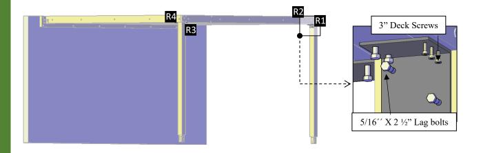
**Step 10:** Use 3" Deck Screws (I) to attach the Tap Angles (12) to the posts and to the Support. Match the number in the Tap angles with the number in the angles.
