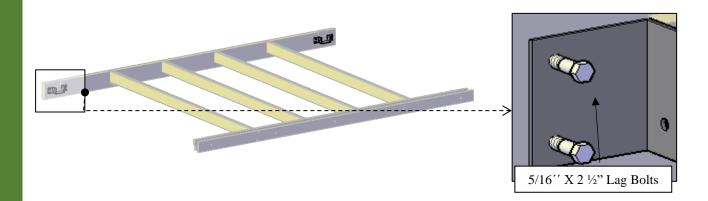
**Step 5:** Use ½" X 6" Anchor Bolts (**K**) (for concrete wall) or 1/2" x 6" Lag Bolts (**G**) (for wood wall) to attach the Ledger Boards (**2**) to the Wall. After that, use 3/8" X 8" bolts (**H**) to attach the Frame to the posts (**1**). Match the number in the top of the post
