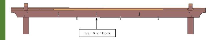
**Step 5:** Attach the perimeter arched rafters (4) to the posts with 3/8" x 7" bolts (C) and to the supports with 8" x 3" deck screws (D). Each part has a series of numbers that indicate where to attach the part with the corresponding number.
