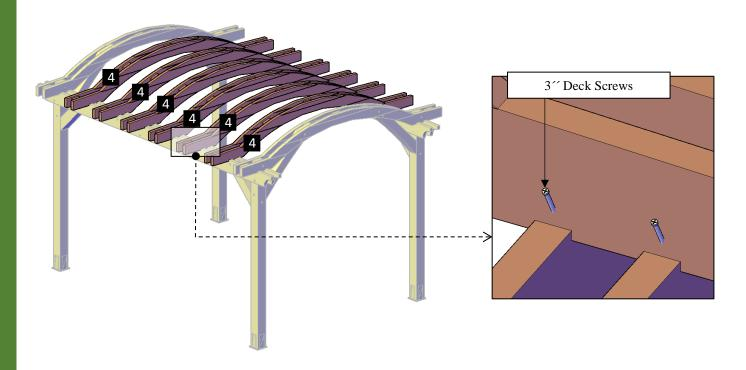
**Step 9:** Use 1 5/8" deck screws (**F**) to attach the roof boards (**7**) to the arched rafters. Each part has a series of numbers that indicate where to attach the part with the corresponding number.
