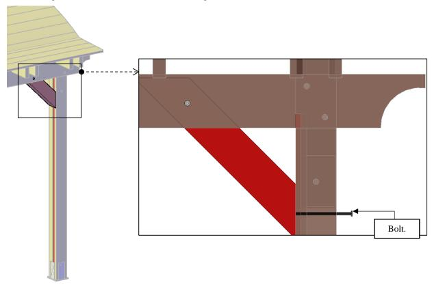
**Step 4:** Swing the brace aside. After that, remove the trim.
