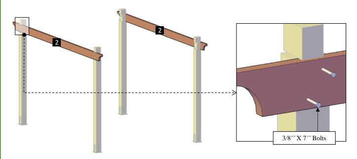
Step 3: Put up the supports with in-between blocking (3), into the post notches as shown and attach to the posts with the single support bolts (C). Each part has a series of numbers that indicate where to attach the part with the corresponding number.
