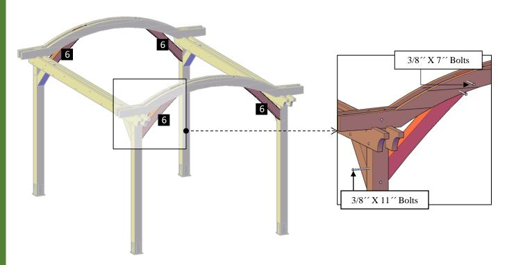
**Step 8:** Use 8" x 3" deck screws (**D**) to attach the other arched rafters (**4**) to the supports. Each part has a series of numbers that indicate where to attach the part with the corresponding number.
