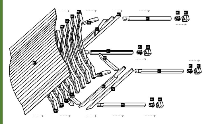
**NOTE:** In order to know where the post needs to be placed, check the numbers on them. If the post is not marked, then place the single Supports on the ground to locate the markings for each post position and clearly set your bearings. ("Don't attach yet, only place them on the ground to begin with").
