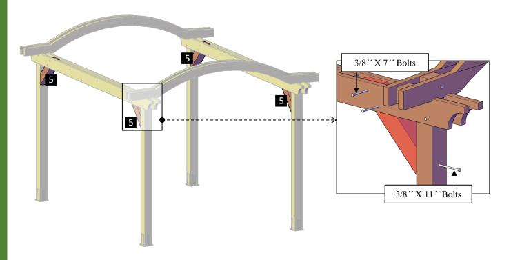
**Step 7:** Attach the secondary knee braces (6) to the posts with 3/8" x 11" bolts (E) and to the arched rafters with 3/8" x 7" bolts (C). Each part has a series of numbers that indicate where to attach the part with the corresponding number.
