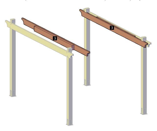
Step 4: Attach the single supports (2) to the supports with in-between blocking (3), use 3/8" X 7" bolts (C). The quantity of bolts depends on the length of the supports.
