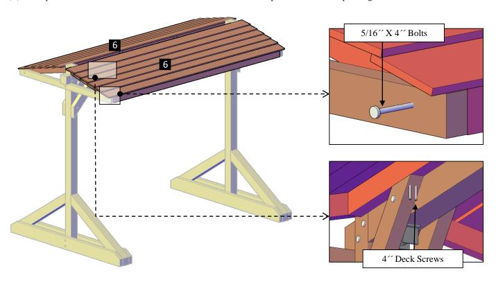
**Step 7:** Use  $2\frac{1}{2}$  deck screws (**G**) to attach the roof board (**7**) to the posts. Each part has a series of numbers that indicate where to attach the part with the corresponding number.
