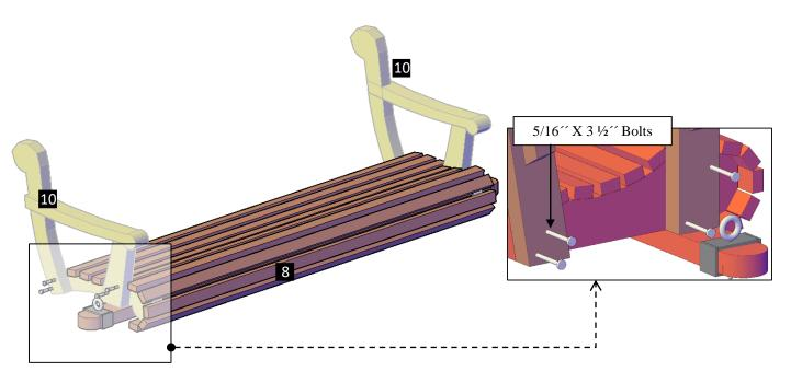
**Step 9:** Attach the backrest **(9)** to the armrest with 5/16" x 3 ½" bolts **(C)** and 3/8" x 3 ½" eyebolts **(H)**. Each part has a series of numbers that indicate where to attach the part with the corresponding number.
