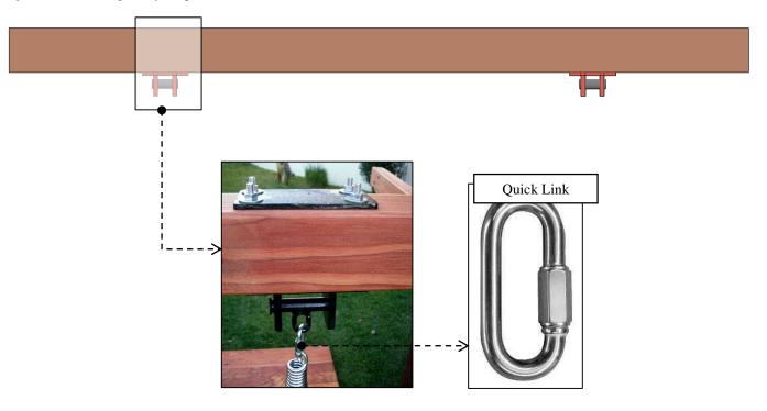
**Step 3:** Use 5/16 'x  $3\frac{1}{2}$  'bolts (C) to attach the support (3) to the posts. Each part has a series of numbers that indicate where to attach the part with the corresponding number.
