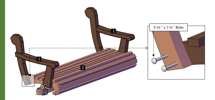
**Step 2:** Attach the backrest (3) to the armrests with 5/16 x  $3\frac{1}{2}$  bolts (A) and 4 x 3/8 eyebolts (B). Each part has a series of numbers that indicate where to attach the part with the corresponding number.
